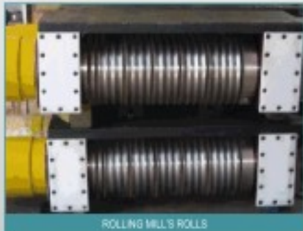
ROLLING MILL'S ROLLS
